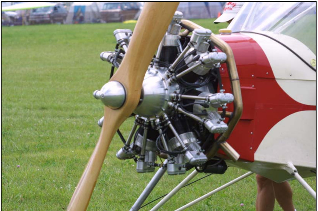
Little Wing 3, converted to the R2800 Rotec Radial engine
